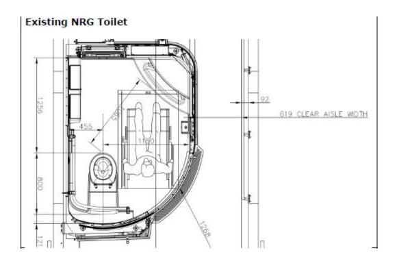
The curved door inhibits the movement of persons using wheelchairs as they manoeuvre inside the toilet. It does not allow a parallel transfer to the toilet pedestal.
